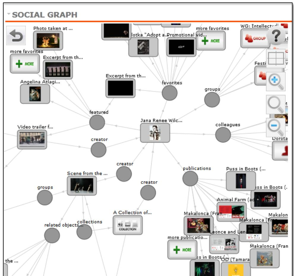
A special node is the **'More'** node that is presented when in a relation are present many nodes (e.g., the content associated with a group). In this case, providing all nodes could be infeasible thus a limited number of nodes is provided and a 'more' node is added to the relation. Clicking on it other nodes are added to the relation in a way similar to classical pagination used to present long lists in HTML.
